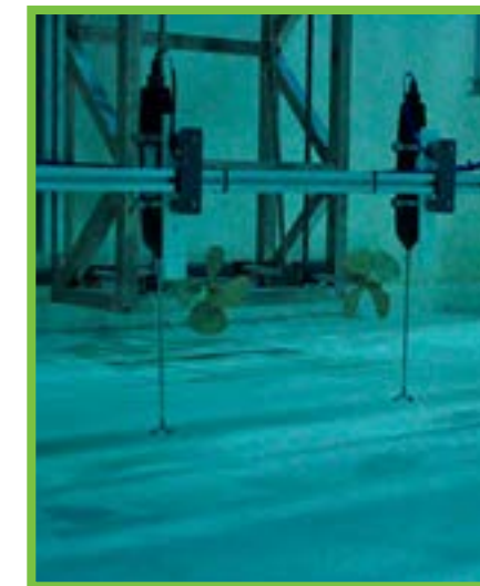
Twin propeller test to study de velocity field generated over a rigid and mobile bottom (@iCIEM).
